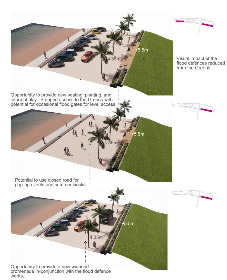
Pier Approach was chosen as a study area due to the varying existing levels creating a higher than standard wall, and the need for a large flood gate to cross the carriageway.
